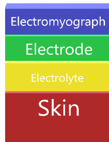
Fig. 3. Diagram of the Electromyograph connection. Own elaboration
